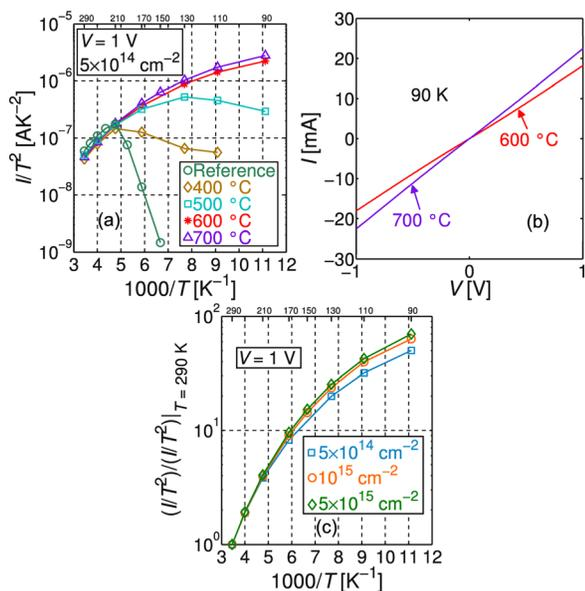
FIG. 2. (Color online) (a) APs for the sample implanted at a dose of  $5 \times 10^{14} \text{ cm}^{-2}$  for all the annealing temperatures, and for a reference sample without implantation. (b)  $I$ - $V$  characteristics of the samples annealed at 600 and 700 °C at 90 K. (c) Normalized APs for the samples annealed at 600 °C for each implanted dose. The APs are displayed for  $V = 1$  V.
