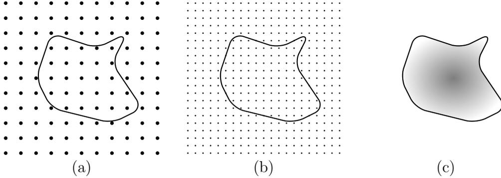
Figure 1: Scaling of a 2D spin lattice: each sub-plot represents the domain  $\Omega$  and (a) the square lattice  $\mathcal{L}$ ; (b) the shrunk square lattice  $\mathcal{L}_2$ ; (c) the homogenized lattice in  $\Omega$  as  $n \rightarrow \infty$ .
