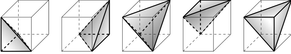
Figure 4: Partition of a single 3D lattice cell. These five tetrahedra are elements  $\mathcal{T}_n$ , and  $T_n$  for the corner tetrahedra, and  $T_n^*$  for the center tetrahedron (see Section 3.3.1).
