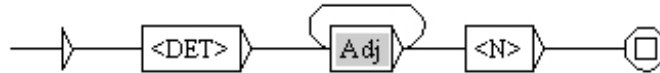
Figure 6.9: Void loop due to a call to a subgraph that recognizes epsilon
