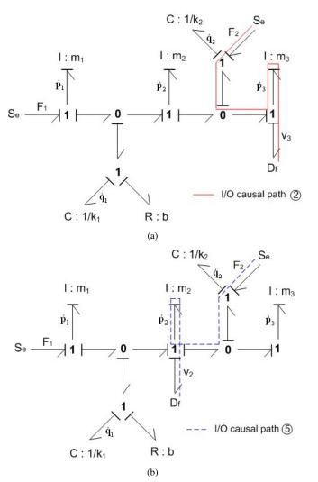
Fig. 13. Determination of infinite zero orders  $\overline{n}_{ij}$ .
