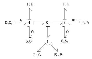
Fig. 4. Example of bicausal bond graph model.
