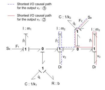
Fig. 12. Determination of the relative orders.
