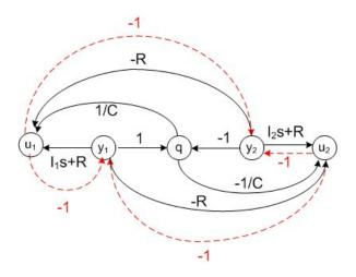
Fig. 2. The digraph  $\mathcal{G}(\Sigma')$  for the determination of the determinant of the system matrix  $\mathbf{P_{inv}}(s)$ .
