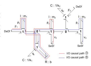
Fig. 15. Determination of essential orders in bicausal bond graph model.
