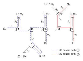
Fig. 9. Set  $S_1$  of different I/O causal paths.
