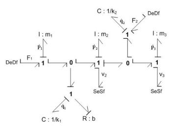
Fig. 10. Bicausal bond graph model of the mechanical system.
