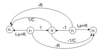
Fig. 1. Example of the digraph representation of an inverse model.
