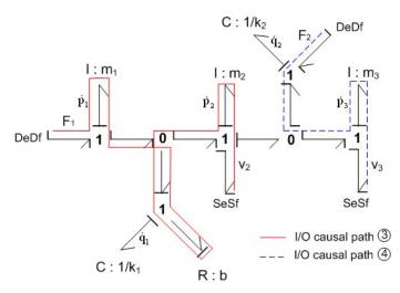
Fig. 11. Set  $S_2$  of different I/O causal paths.
