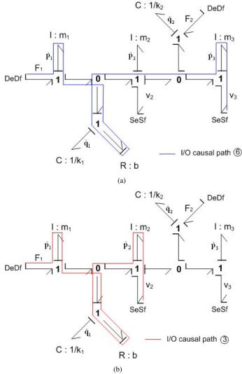
Fig. 14. Determination of infinite pole orders  $\overline{n}_{ij}$ .
