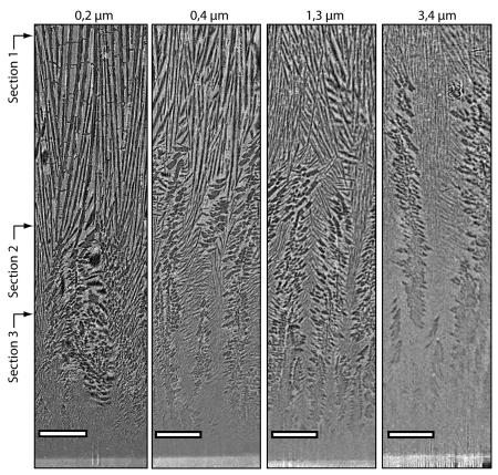
Figure 2: Initial transition zone, influence of particles size. Scale bars 250  $\mu$ m. Vertical cross-sections. Sections 1-3 refer to cross-sections in figure 3.
