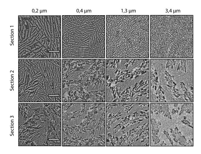
Figure 3: Initial transition zone, influence of particles size. Scale bars 150  $\mu$ m. Horizontal cross-sections. The different sections are defined in figure 2. The cohabitation of r- and z-crystals (see reference <sup>4</sup> for definition) during the initial instants is clearly visible.
