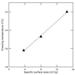
Figure 4: Freezing temperature vs. specific surface area. The nucleation temperature for the 3.4  $\mu m$  powder is not available.
