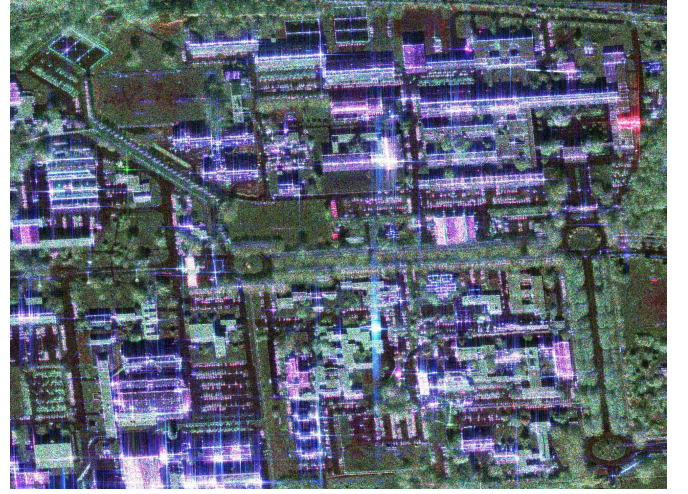
Fig. 1. Toulouse, RAMSES POLSAR data, X-band, 1500 \times 2000 pixels: amplitude color composition of the target vector elements k_1 - k_3 - k_2 .
