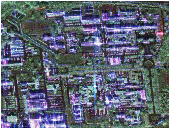
Fig. 2. Toulouse, RAMSES POLSAR data, X-band, 1500 \times 2000 pixels: amplitude color composition of the target vector elements k_1 - k_3 - k_2 .
