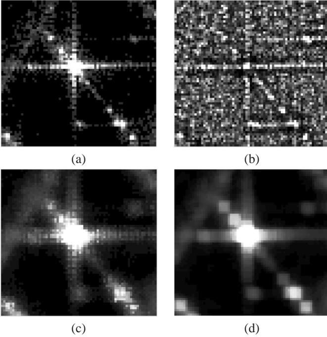
Fig. 3. Toulouse, RAMSES POLSAR data, X-band,  $50 \times 50$  pixels, zoom image: (a) FP-PWF texture, (b) SCM-PWF normalized texture, (c) span estimated using  $\widehat{\sigma}_0$  from Eq. 9 and (d) SCM-MPWF span.
