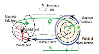
Figure 4: Position coordinates in use in a Tokamak. (Source: V. Grandgirard's Lectures at Cemracs'10).
