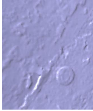
Figure 5: Detail of the 3D model of the wall painting in Rudesheim. The approximately 0.1 mm thick photogrammetric target is observable.
