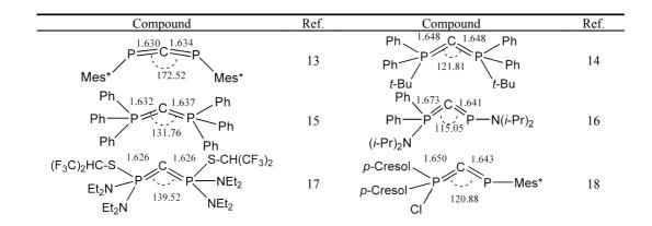
**Table 2**Relevant geometrical parameters determined through X-ray diffraction on linear P-C-Psystems
