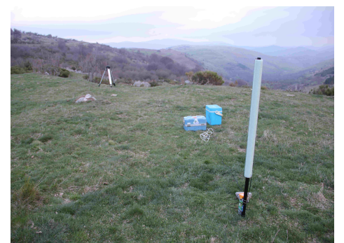
From left to right: VHF aerial, electronics container and ELF/VLF aerial
