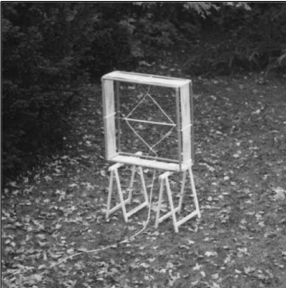
Fig 7: 137kHz receiving loop antenna.
