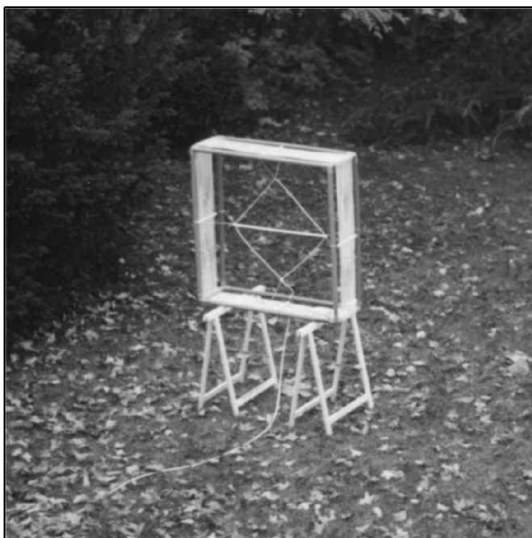
Fig 7: 137kHz receiving loop antenna.
