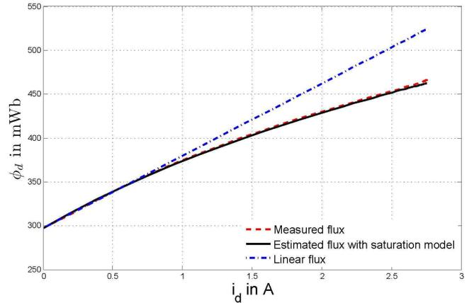
Fig. 7. Saturation curve  $\phi_d - i_d$  (IPM).
