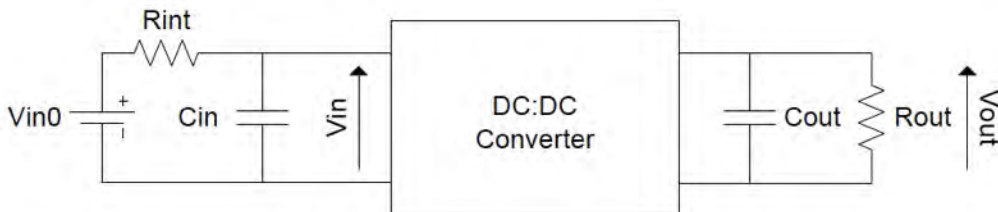
Fig. 10: Test of harvesting converters with MFCs basic electrical model
