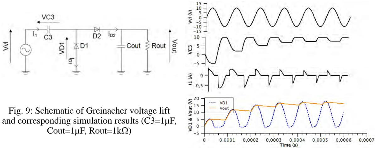
Fig. 9: Schematic of Greinacher voltage lift and corresponding simulation results ( $C_3=1\mu\text{F}$ ,  $C_{out}=1\mu\text{F}$ ,  $R_{out}=1\text{k}\Omega$ )
