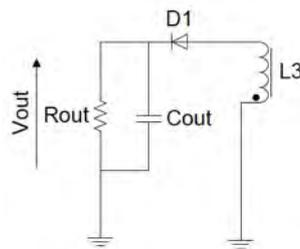
Fig. 7: Output winding schematic of flyback converter (top2).
