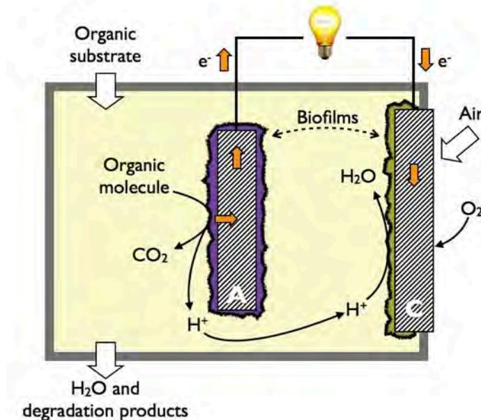
Fig. 1: Schematic diagram of a single chamber MFC
