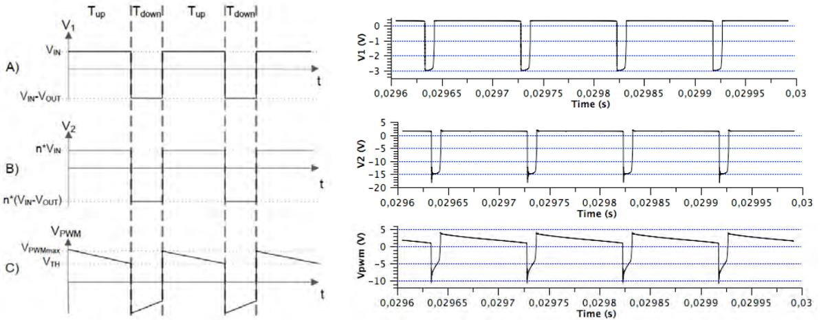
**Fig. 6: Ideal and simulated signals for top1**
