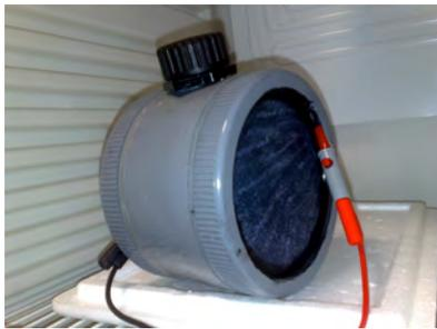
Fig. 2: Picture of 1-liter laboratory MFC
