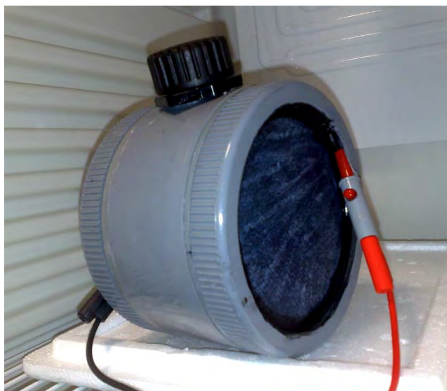
Figure 3. Photograph of the constructed MFC
