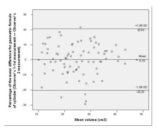
Figure 3b. Bland-Altman plot for the percentage of the mean difference for geometric formula of cylinder (Observer's 1-1st measurement – Observer's 2 measurement) and 95% limits of agreement for interobserver measurements.
