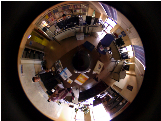
Figure 9: Omnidirectional camera mounted on mobile robot and the real image that it gives
