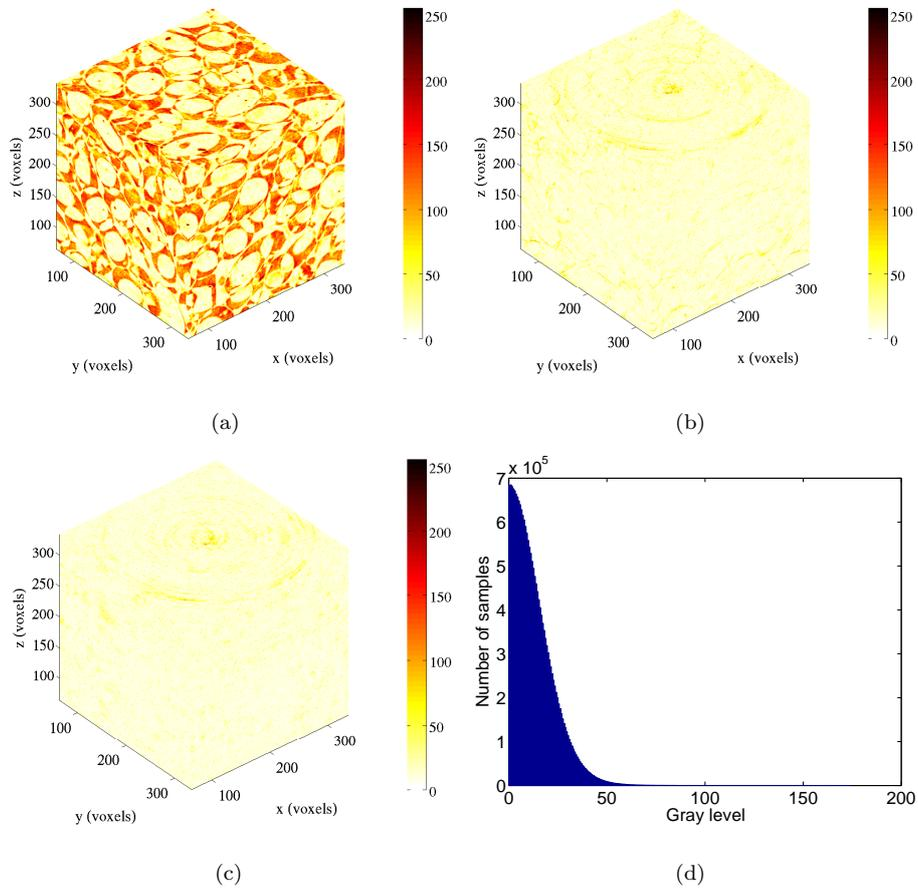
Figure 5: Initial (a), with rigid body translation correction (b), and at convergence (c) correlation residuals  $|f - g|$  when the volume of the first load level is registered with the reference. Gray level histogram of the residuals  $|f - g|$  at convergence to be compared with that shown in Figure 2(b).
