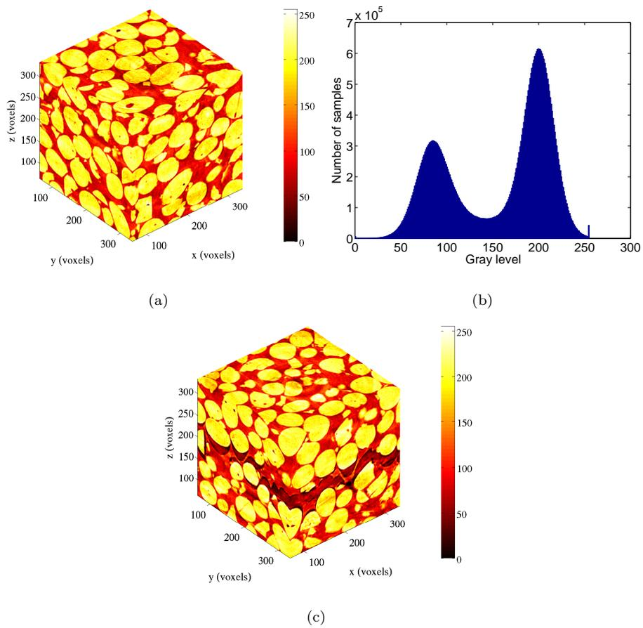
Figure 2:  $272 \times 272 \times 272$ -voxel ROI (8-bit digitization) of the analyzed propellant in its reference configuration (a), and after failure (c). Note that the failure plane can be seen in the latter volume as a darker zone. Gray level histogram (b) of the reference ROI.
