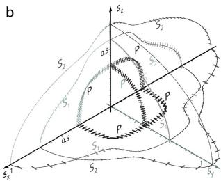
FIG. 4. Intersection of the slowness surfaces of the normally polarized medium (a) and anomalously polarized medium (b) with the coordinates planes. The normally polarized medium corresponds to the stiffness matrix (25). The polarization vectors are indicated. Anomalous polarization occurs in the (x, y)- and (x, z)-planes. The angle between the qP polarization and the propagation direction goes beyond  $\pi/2$  in the midrange of the two planes (close to the letter "P").
