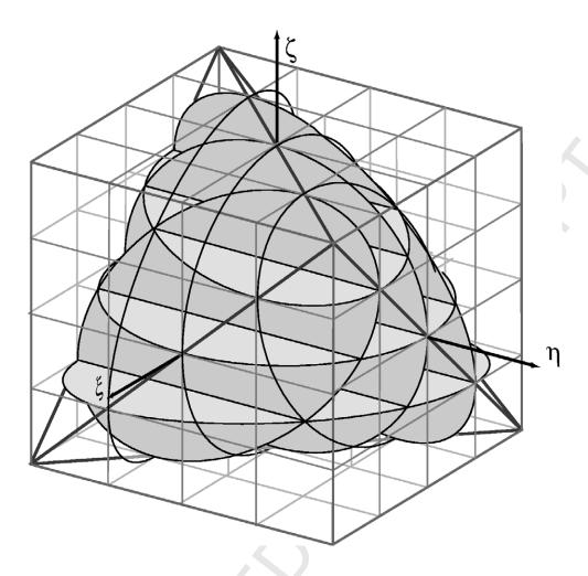
FIG. 1. An orthorhombic medium is stable if the "diagonal" stiffness components are positive and if the variables  $\xi = c_{23}/\sqrt{c_{22}c_{33}}$ ,  $\eta = c_{13}/\sqrt{c_{11}c_{33}}$  and  $\zeta = c_{12}/\sqrt{c_{11}c_{22}}$  satisfy the four inequalities  $\xi^2 < 1$ ,  $\eta^2 < 1$ ,  $\zeta^2 < 1$ , and  $2\xi\eta\zeta - \xi^2 - \eta^2 - \zeta^2 + 1 > 0$ , i.e., if the point  $(\xi, \eta, \zeta)$  lies inside the stability volume (the "tetrahedral cushion").
