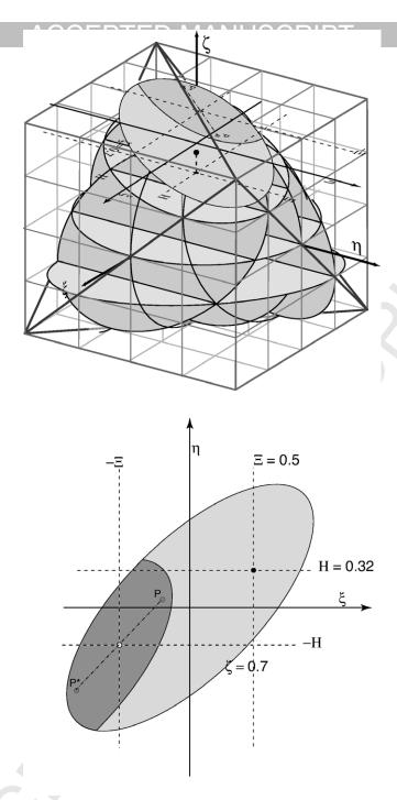
FIG. 2. Intersection of the stability volume of the original medium with that of the anomalous companion medium is shown for the plane  $\zeta=0.7$ . The intersection is non-empty if - and only if - the point  $(\Xi,H,\zeta)$  lies within the original stability volume.
