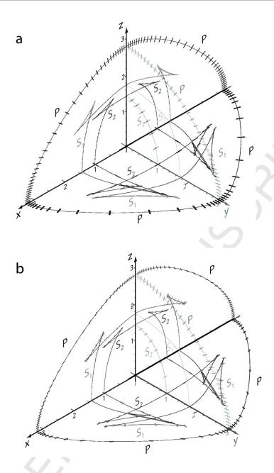
FIG. 5. Intersection of the wave (ray) surfaces of the normally polarized medium (a) and anomalously polarized medium (b) with the coordinates planes. The normally polarized medium corresponds to the stiffness matrix (25). The polarization vectors are indicated. Anomalous polarization occurs in the (x, y)- and (x, z)-planes. The angle between the qP polarization and the propagation direction goes beyond  $\pi/2$  in the midrange of the two planes (close to the letter "P").
