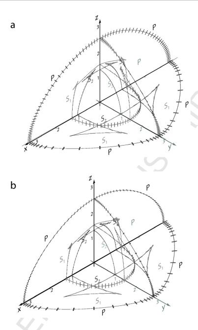
FIG. 7. Intersection of the wave (ray) surfaces of the medium defined by the stiffness matrix (26) (a) and that of the companion medium (b) with the coordinates planes. Polarization vectors are indicated. Note that in (a) the polarization is anomalous in the (y, z)-plane. Anomalous polarizations should occur in the (x, z)- and (y, z)-planes. However, note that in the (y, z)-plane the polarization has changed to normal, while in the (x, z)-plane it is now anomalous.
