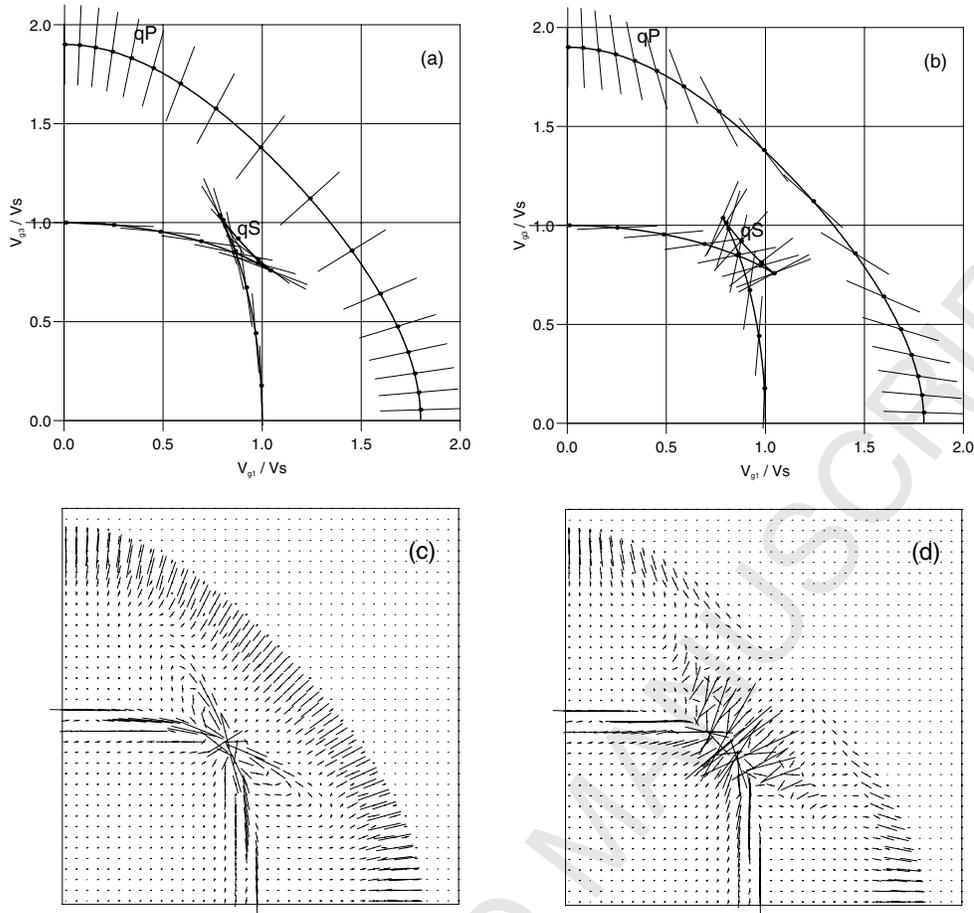
FIG. 3. Normalized ray velocity sections and snapshots for a transversely isotropic medium. Figures (b) and (d) correspond to the anomalous medium.
