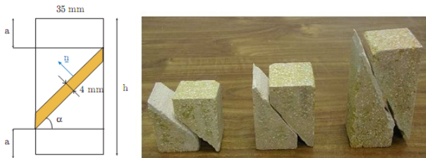
Figure 6 : Compression/shear tests for different angles (45, 55 and 65°). Specimens after failure.
