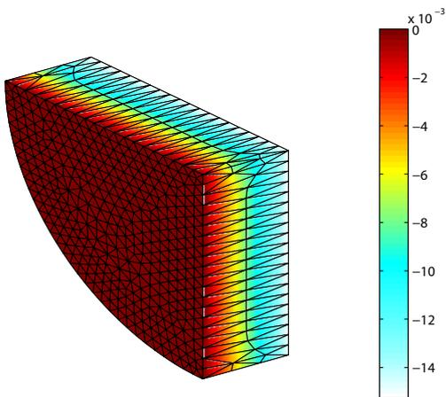
**Fig. 12.** Electric potential for the cylindrical sensor (V).
