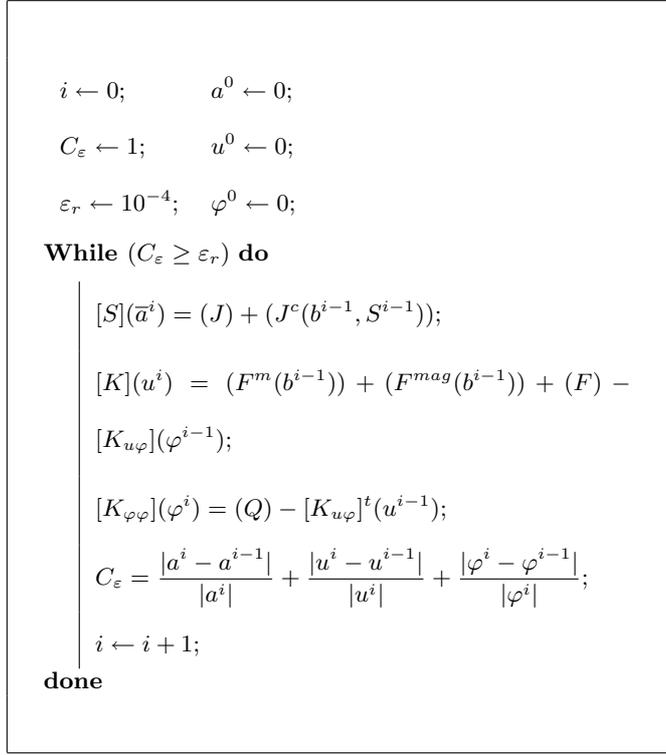
**Fig. 1.** Fixed-point algorithm; *i* represents the iteration number, ε<sub>*r*</sub> the error criterion.
