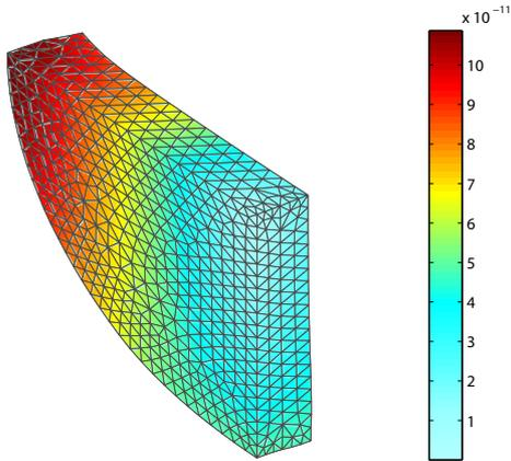
**Fig. 11.** Mechanical displacement for the cylindrical sensor (m).
