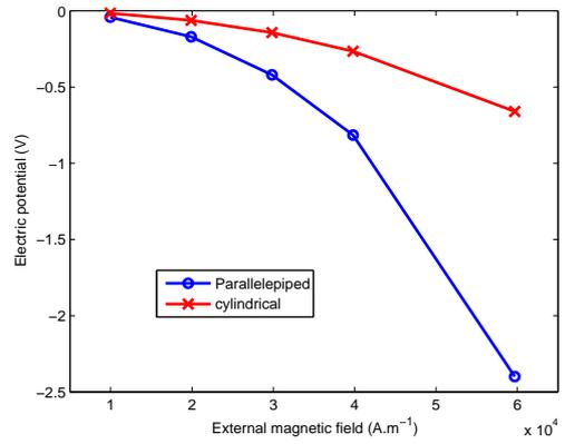
**Fig. 13.** Electric potentials versus external magnetic field.
