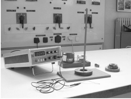
Fig. 3. Our measurement station (model 912 gaussmeter RFL Industries Inc. ).
