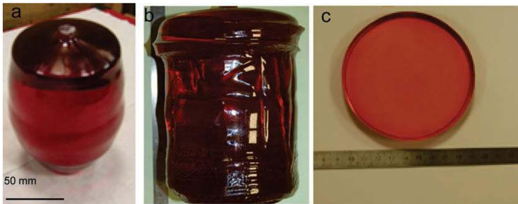
Figure 2. Sapphire ingots grown by the Kyropoulos technique: (a) *a*-axis; (b) *c*-axis; (c) wafer thickness 20 mm.
