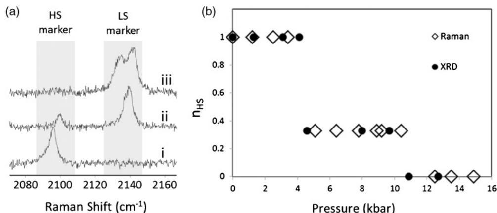
FIG. 3. (a) Raman spectra of compound **1** in the cyano-stretching region at (i) 2.5, (ii) 7.8, and (iii) 13.5 kbar, highlighting the characteristic peaks for the HS and LS molecular spin states. (b) Evolution of the HS fraction in a single crystal of **1** under compression obtained from high-pressure Raman and x-ray diffraction (XRD) data.
