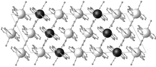
FIG. 5. Extended structure of **1** at 4.6 kbar perpendicular to the *ac*-plane revealing the long-range [HS-LS-LS] order of this pressure-induced intermediate phase. Iron atoms are shown as large spheres, for illustrative purposes. LS Fe atoms are colored white, and HS Fe atoms are colored black. All other atoms are shown as small grey spheres. Hydrogen atoms have been omitted for clarity.
