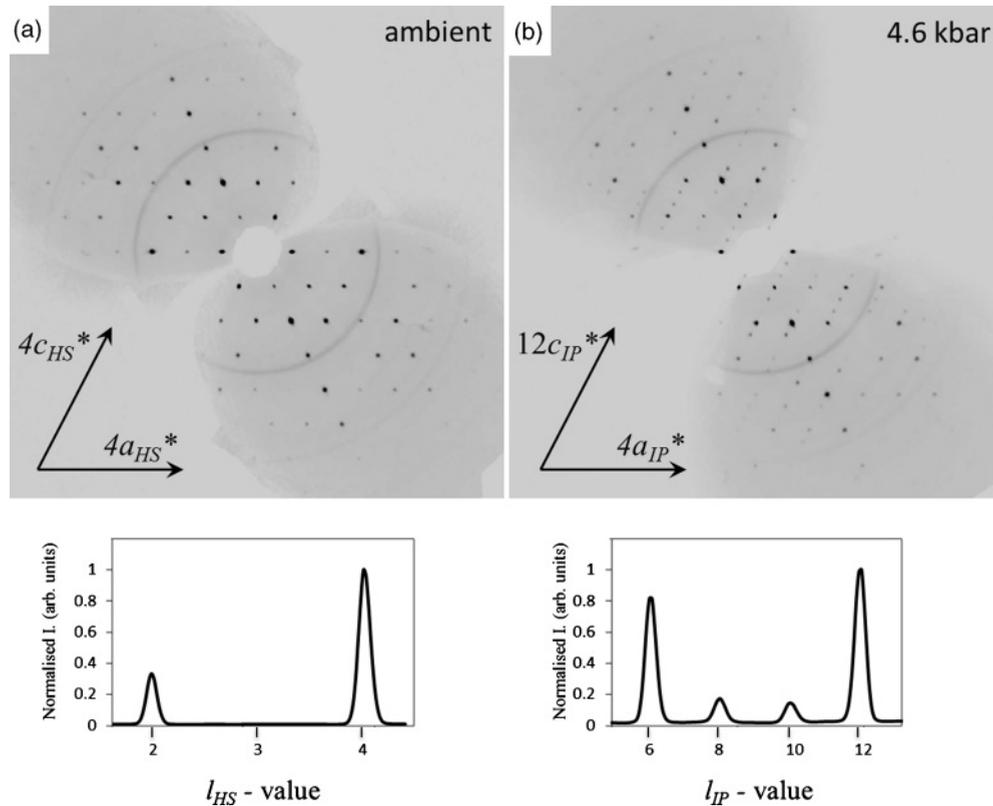
FIG. 4. Pseudoprecission images of the reciprocal lattice in the  $(h0l)$  plane for **1** at (a) ambient pressure (inside the DAC) and (b) 4.6 kbar, reconstructed from the collected diffraction images. For illustrative purposes a plot of normalized intensity along  $(-6,0,l)$  for values of  $l$  between 2 and 4 in the ambient pressure setting is also shown for each image.
