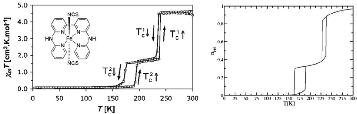
FIG. 1. Molecular structure of  $[\text{Fe}(\text{babppy})(\text{NCS})_2]$  (**1**) and its two-step thermal spin transition curve at atmospheric pressure. Left panel: experimental data and right panel: curve simulated using the Ising-like Hamiltonian with three coupled sublattices proposed in Ref. 19.
