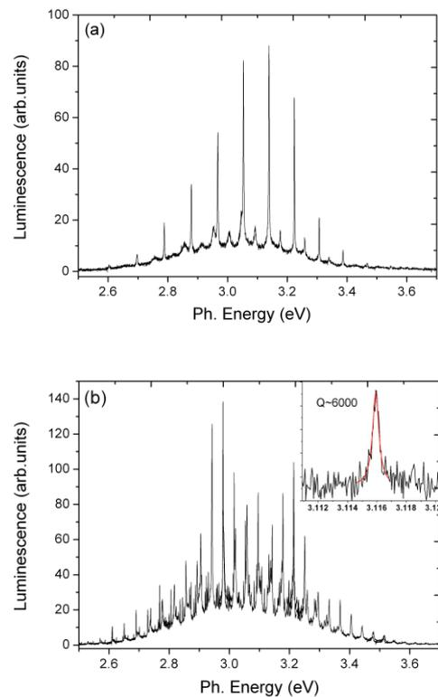
**Figure 2** Photoluminescence spectra of a (a) 2  $\mu\text{m}$  and (b) 5  $\mu\text{m}$  in diameter microdisk. Inset : High resolution spectrum of a WGM of high Q value, i.e.  $Q \sim 6000$ ; the peak is fitted by a Lorentzian line shape (red line).
