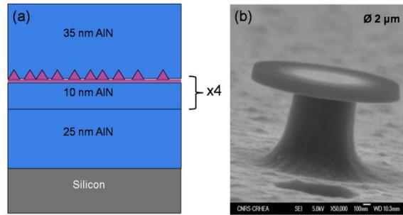
**Figure 1** a) Epitaxial structure : the optically active area above the Silicon substrate contains 4 periods of GaN/AlN QDs layers. b) Scanning Electron Microscopy image of a 2  $\mu\text{m}$  in diameter microdisk.
