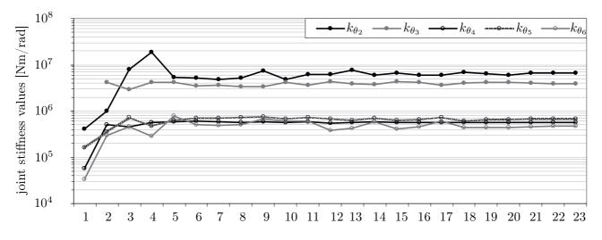
Figure 7: Influence of the number of tests on the joint stiffness values evaluation
