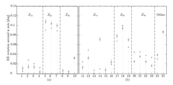
Figure 10: Calculated and measured rotations of the EE expressed around  $\mathbf{x}$  axis of  $\mathcal{F}_0$ : (a) Validation with the tests used for the joint stiffness identification; (b) Validation with the other tests
