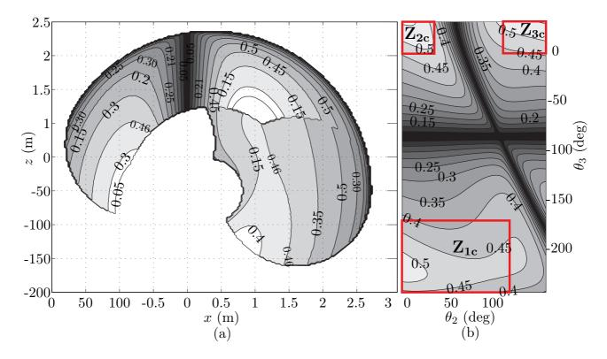
Figure 3: Contours of the inverse condition number of  $\mathbf{J}_N$ : (a) in the robot Cartesian workspace and (b) in the joint space  $(\theta_2, \theta_3)$
