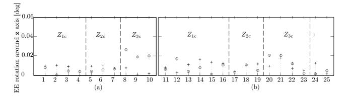
Figure 12: Calculated and measured rotations of the EE expressed around  $\mathbf{z}$  axis of  $\mathcal{F}_0$ : (a) Validation with the tests used for the joint stiffness identification; (b) Validation with the other tests
