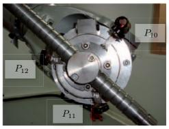
Figure 6: Robot end-effector and location of points  $P_{10}$ ,  $P_{11}$  and  $P_{12}$
