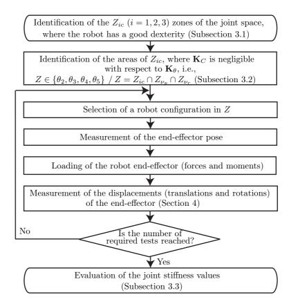
Figure 2: Procedure for the joint stiffness identification
