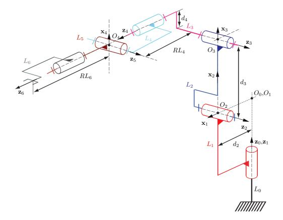
Figure 1: DHm Parameterization of the Kuka KR240-2 robot
