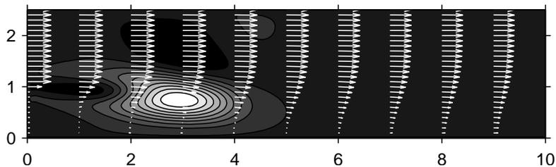
Figure 1: Arrows: velocity vectors of a confined wake flow at  $Re = 100$ . Contours: the structural sensitivity of this flow, calculated with a local stability analysis.
