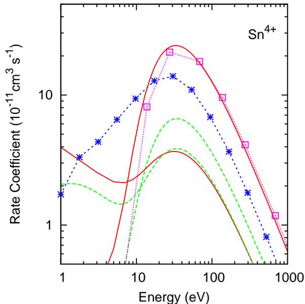
**Figure 15.** Total dielectronic recombination rate coefficients for  $\text{Sn}^{4+}$ : where there are pairs of curves the lower/upper are with/without  $n = 5$  (see text). Solid (red) curves: configuration-average; long-dashed (green) curves: AUTOSTRUCTURE averaged over the initial ground level; short-dashed (blue) curve: Burgess–Bethe General Program averaged over the initial ground level; dotted (purple) curve; Burgess General Formula. All this work.
