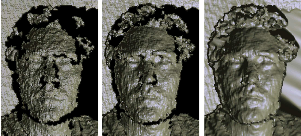
Left: raw data from a single frame. Middle: temporally smoothed data. Right: additionally Gauss-filtered data 187x84mm (600 x 600 DPI)
