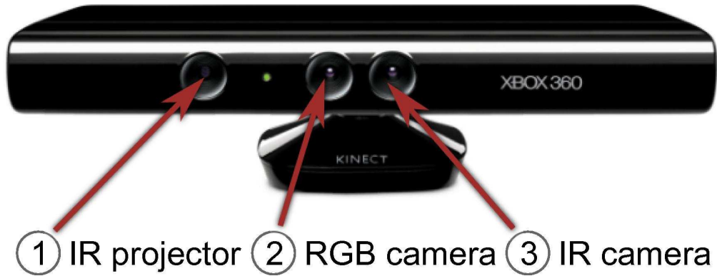
Microsoft Xbox Kinect sensor 72x28mm (600 x 600 DPI)
