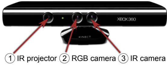
Figure 2: Microsoft Xbox Kinect sensor
