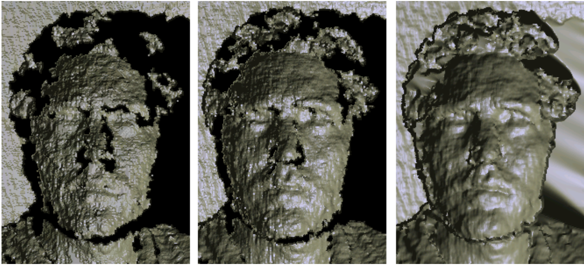
Figure 3: Left: raw data from a single frame. Middle: temporally smoothed data. Right: additionally Gauss-filtered data
