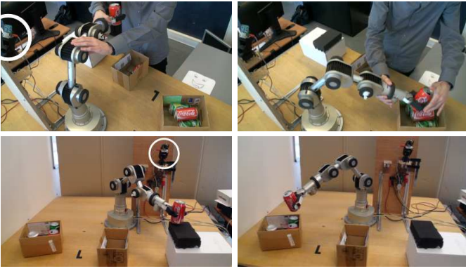
Fig. 3. Pick-and-place task learned and adapted through passive manipulation. Example of demonstration for the red-can-in-box-2 condition and reproduction by the robot. The camera looks at the pick-up place to recognize the type of object by color detection (red or green).
