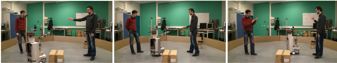
Figure 4: Obstacle avoidance while reaching for a pink ball held by a human interacting with the robot.
