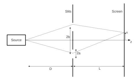
FIG. 1. Schematic depiction of the apparatus with the source, the two-slits and the screen and hence,
