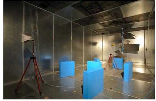
Fig. 6. Experimental configuration with  $N = 6$  pieces of absorbers
