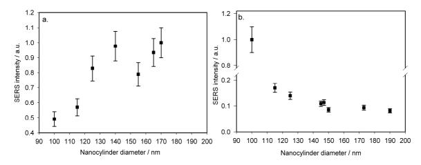
Figure 2. SERS intensity as a function of the nanocylinder diameters: (a) for the BSA Raman bands located at 1614 and 1658 cm<sup>-1</sup> and (b) for the RNase-A Raman band located at 1614 cm<sup>-1</sup>. In order to make more readable the errors bars in figure 2(b) we applied a break on the Y axis (between 0.22 and 0.78)
