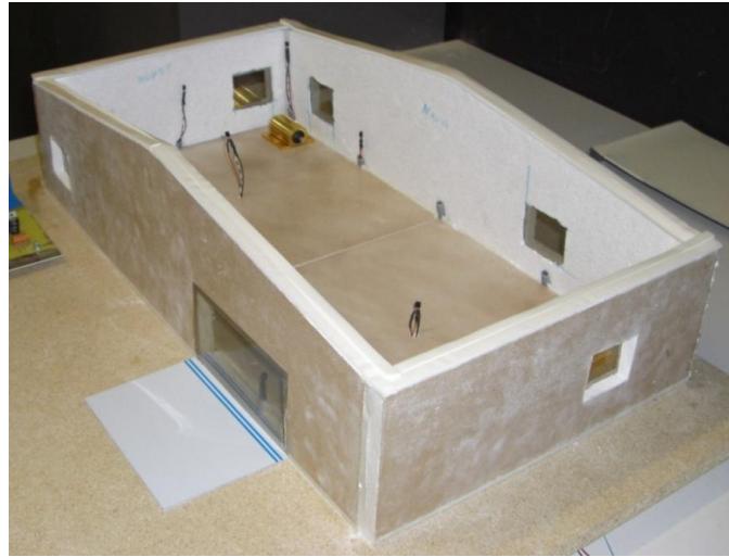
Figure 2. The building mock-up used for testing the proposed hybrid control scheme.
