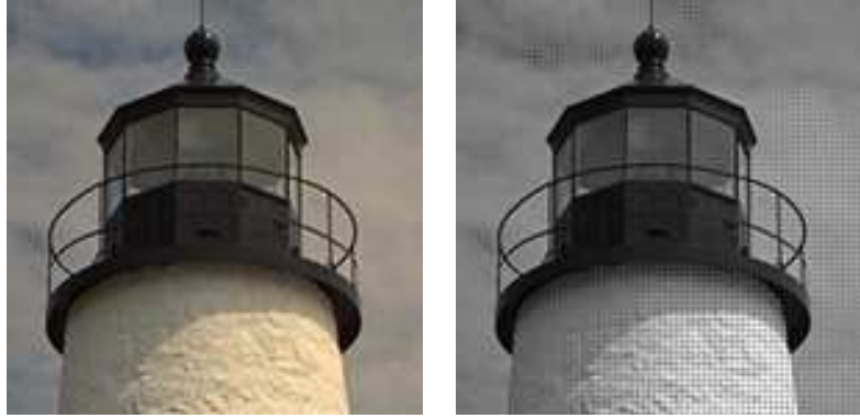
Figure 2. Bayer CFA-based single-sensor imaging: (a) full-color image and (b) grayscale CFA image.
