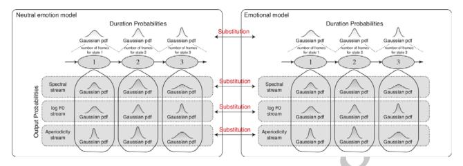
Figure 1: Substitution of each component in an HMM-based speech synthesis system. This enables separate assessment of the importance of spectral and prosody components for emotional speech.
