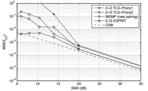
**Fig. 2.** Performance comparison of the 2-D ESPRIT, MEMP, TLS-Prony1–2 algorithms. Identical and close modes in each dimension.
