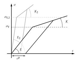
Figure 5: Plasticity constitutive laws controlling the ductility of the abradable coating
