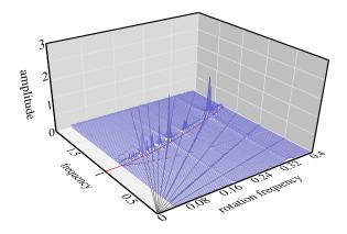
Figure 15: Blade spectrum with tangential efforts for E = 10 and K = 4.55
