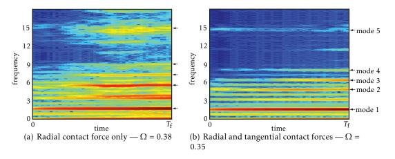
Figure 16: Spectrograms of the blade response
