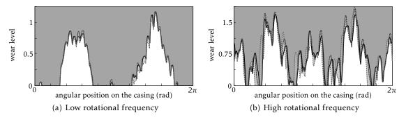
Figure 7: Final abradable profiles for two densities after twenty rounds of the blade
