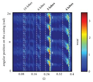
Figure 14: Abradable coating wear patterns
