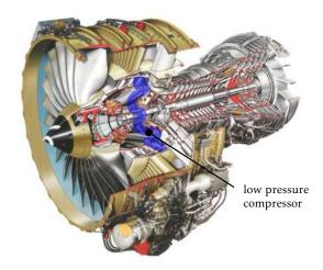
Figure 1: Low pressure compressor. Courtesy of CFM International
