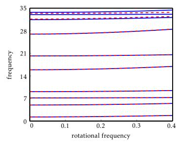
Figure 3: Campbell diagrams with centrifugal stiffening: reduced-order model (--) and full finite element model with no parametrization of the stiffness matrix (--)
