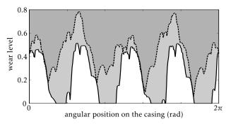
Figure 12: Final abradable profiles for E = 1 ( $\longrightarrow$ ) and E = 10 ( $\frown$ ) at respective critical rotational frequency for k = 4 after twenty rounds
