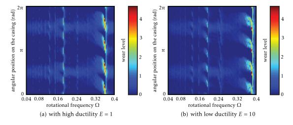
Figure 11: Maps of the final abradable profiles with respect to  $\Omega$  for interface node 1 after twenty rounds of the blade
