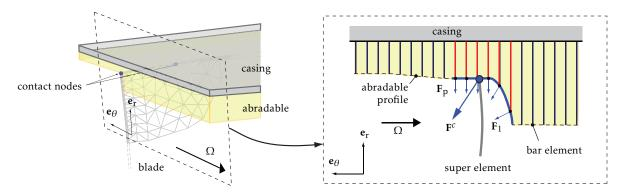
Figure 4: Blade interface node and associated geometrical profile
