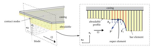
Figure 4: Blade interface node and associated geometrical profile
