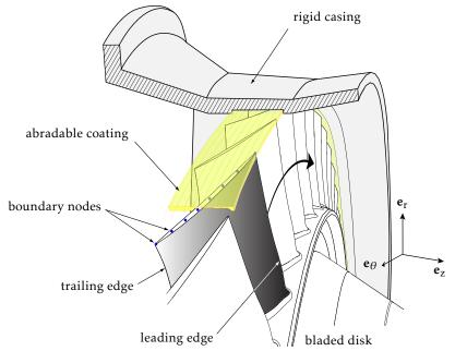
Figure 2: Blade under investigation with eight anticipated boundary nodes undergoing contact constraints and abradable removal conditions
