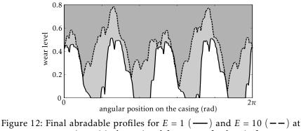
Figure 12: Final abradable profiles for E = 1 (---) and E = 10 (--) at respective critical rotational frequency for k = 4 after twenty rounds
