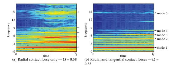
Figure 16: Spectrograms of the blade response
