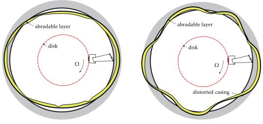
(a) Multi-harmonic 2-nodal diameter distortion (b) Coupled 2- and 5-nodal diameter distortion
