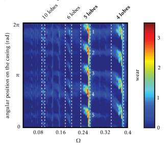
Figure 14: Abradable coating wear patterns
