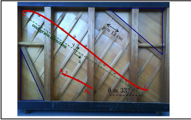
Figure 1. Rear view of the upright piano studied with the wood grain direction added in green and the two bridges (on the other side of the soundboard) added in red.
