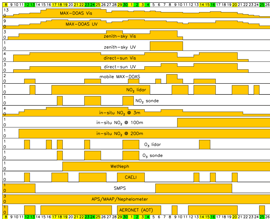
Fig. 9. Number of instruments which have collected data on each day during the CINDI campaign and for each of the instrument types. The day numbers in June and July are at the top and bottom of the figure. The yellow and green days are days of category A and B, respectively (see Sect. 3.1).
