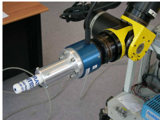
Fig. 6. End-effector used for the "Go and write" mission.
