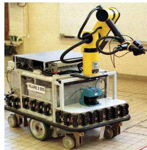
Fig. 2. H_2bis : a 3-dimensional mobile manipulator.
