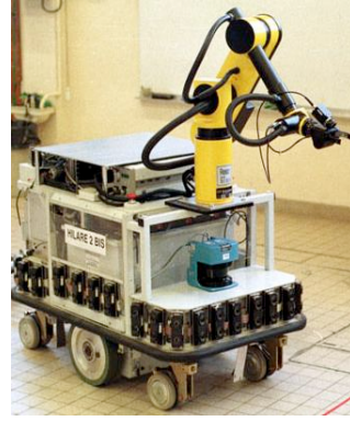
Fig. 1. H2bis : a 3-dimensional mobile manipulator.
