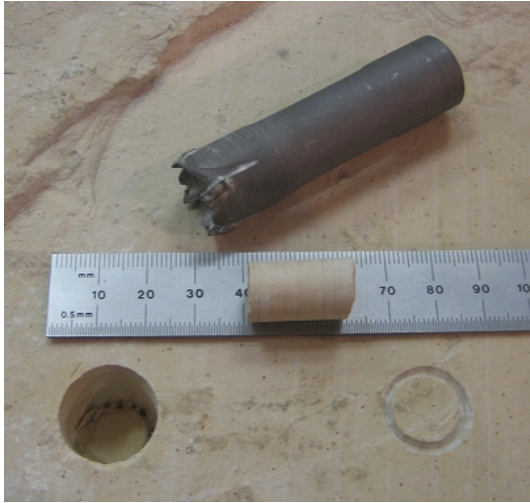
Figure 7: Coring Bit and Resulting Hole and Core
