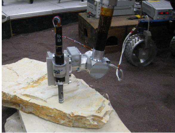
Figure 3: Percussive coring test
