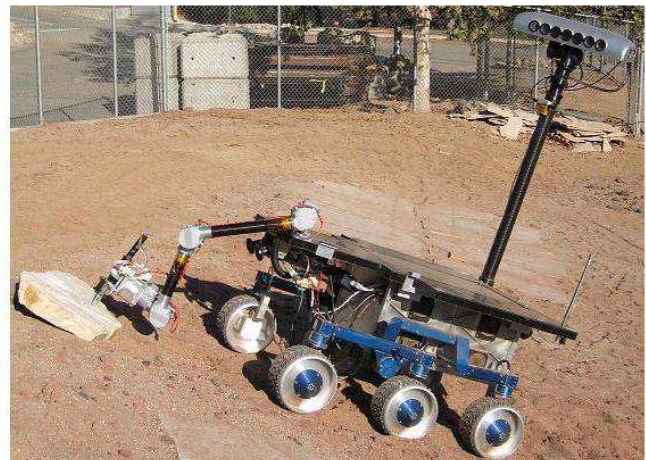
Figure 1: Coring on a 26 degree slope in the Marsyard
